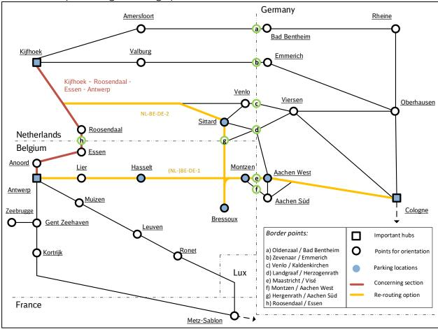
This is a double mixed (passenger and freight trains) track. In the Netherlands it has ATB signalling and 1,5 kV electricity. In Belgium (as from Roosendaal) it has TBL1+ signalling and 3 kV electricity.
