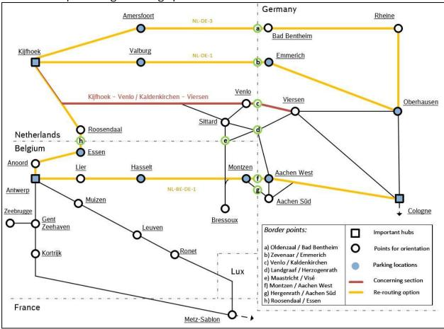
For the Netherlands, the route via Venlo / Kaldenkirchen is the second main freight route to Germany. It is a double mixed track (passenger and freight trains) with ATB signalling and 1,5 kV electricity. Between Kaldenkirchen and Viersen Gbf it is a single track, with PZB and 15 kV.
