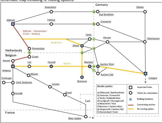
This is a double mixed (passenger and freight trains) track. In the Netherlands it has ATB signalling and 1,5 kV electricity. In Belgium (as from Roosendaal) it has TBL1 signalling and 3 kV electricity.
