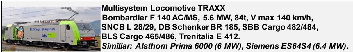
Figure 6: Multisystem locos TRAXX running on Corridor Rotterdam-Genoa.
