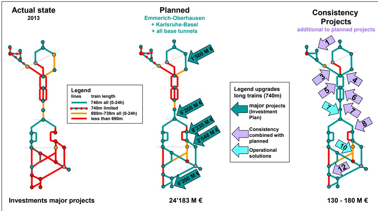
Figure 17: Development of topology for long trains with planned projects, consistency projects and operational solutions.
