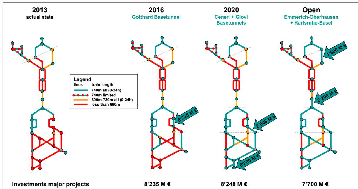
Figure 12: Development of topology for long trains with investment plan of Table 2.
